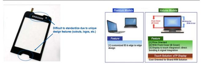
Figure 7. Touchscreen module for mobile device
