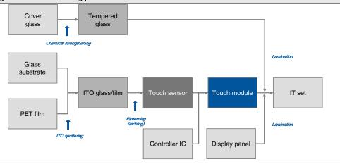
Figure 50. Manufacturing process for add-on touchscreens
