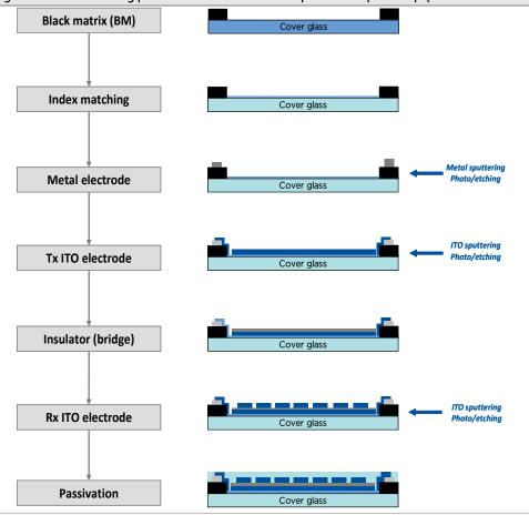
Figure 56. Manufacturing process for OGS touchscreen panels with photo equipment
