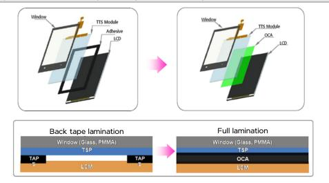
Figure 58. Comparison of air gap bonding and direct bonding (full lamination)
