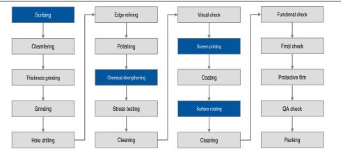
Figure 53. Manufacturing process for cover glass
